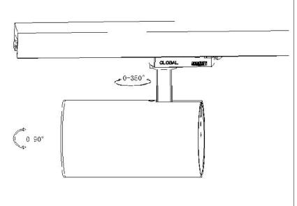
Step 5: Adjust the right angle and connect electricity
