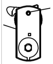
Step 3: For the lock switch and scroll lock, before installation, make sure it's in the status as below. Lock switch on the left and scroll lock should be in "0".
