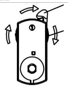
Step 4: Attach the adaptor on the track, turn the lock switch to the right as indicated. Scroll the scroll lock to the designated circuit.
